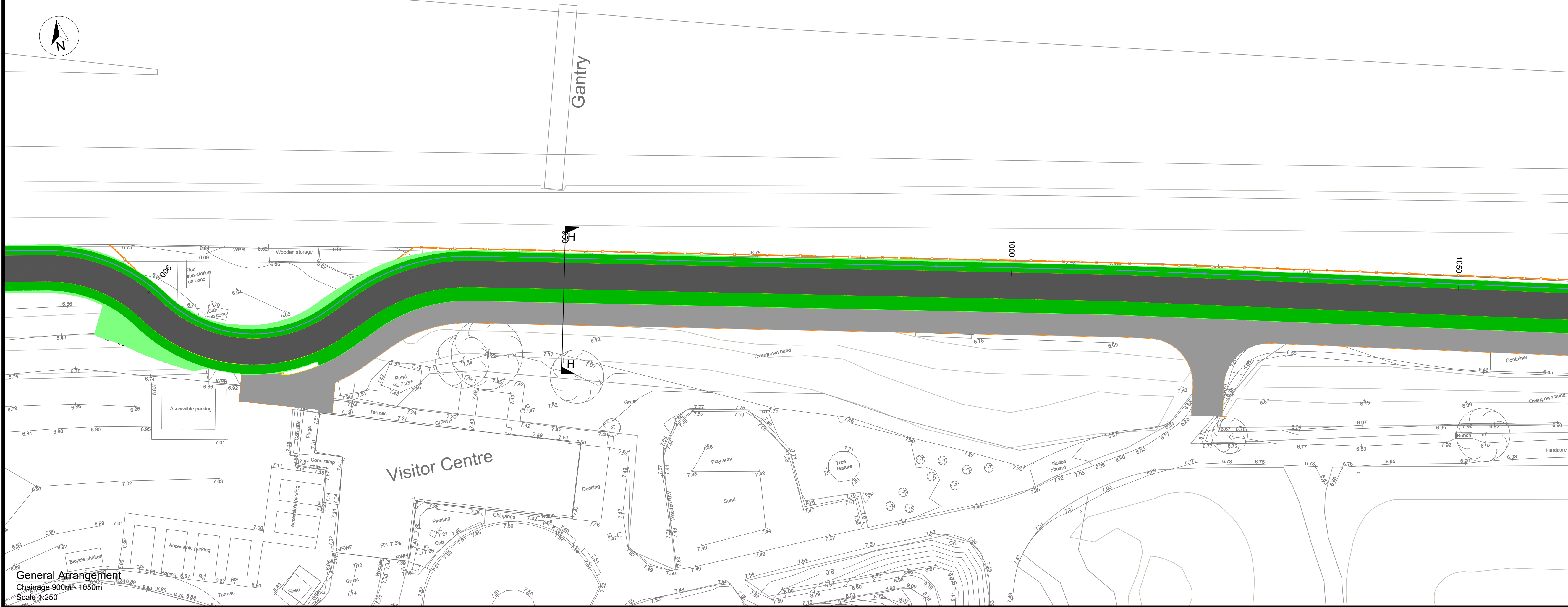
General Arrangement Chainage 750m - 900m Scale 1:250
